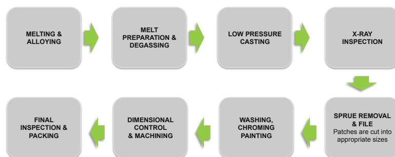
Figure 3: A process flow diagram 3 for the production of aluminum wheels by low-pressure casting
